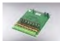
5201 8 fire detection lines
